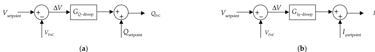
Figure 4. Proportional control based reactive power control strategy at smart converter: (a) Voltage Q-droop control; (b) Voltage I_q -droop control.
